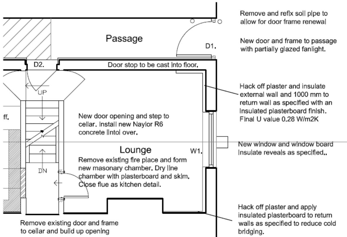
Note that internal insulation has been applied to the front and external insulation within the passageway, creating minimal obstruction to internal doors and circulation space around the stairway.
