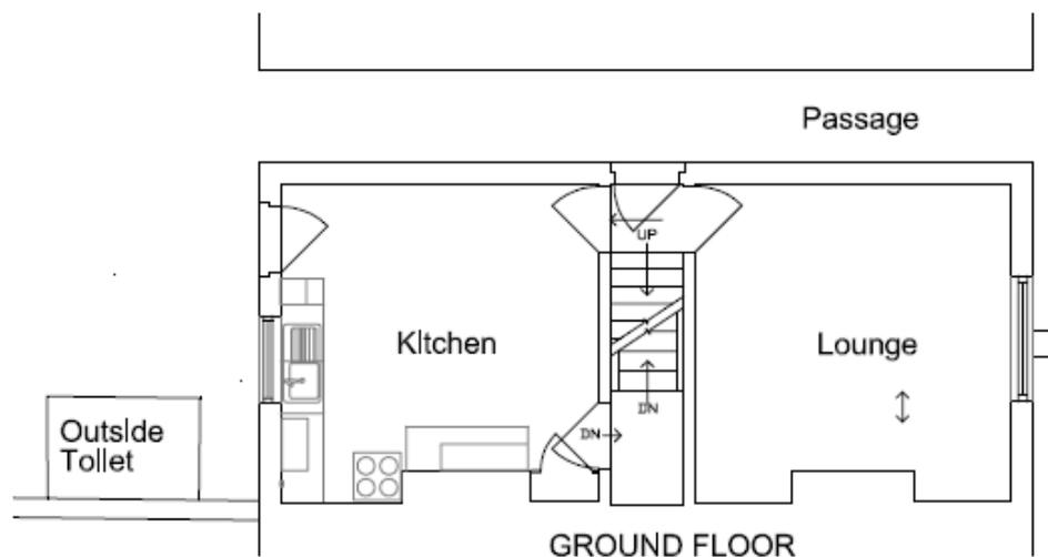
While front wall insulation can be done internally with little loss of space. Insulation of solid wall passages, as with end walls, may need to be done externally. This insulation should be both of the wall and the floor over the passageway.
