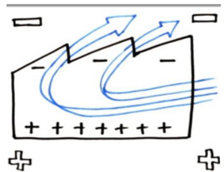
Lower air pressures at higher heights can passively pull air through a building.
