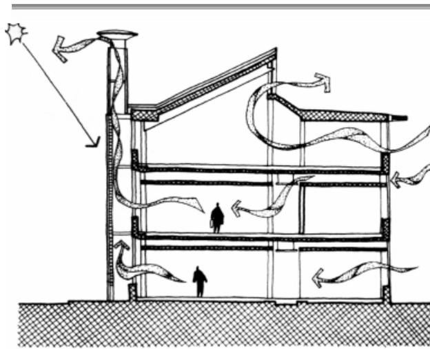
The stack effect: hot air rises due to buoyancy, and its low pressure sucks in fresh air from outside
